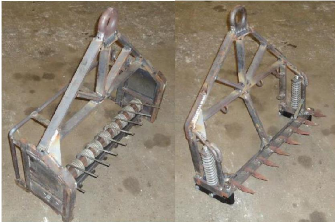
Figure 5: The N-Virodredge design (left) separate from the steel belly bag, with individually sprung tines and side skids; compared to the Newhaven dredge (right) with a fixed tooth bar. Source: Filippi, (2013).
