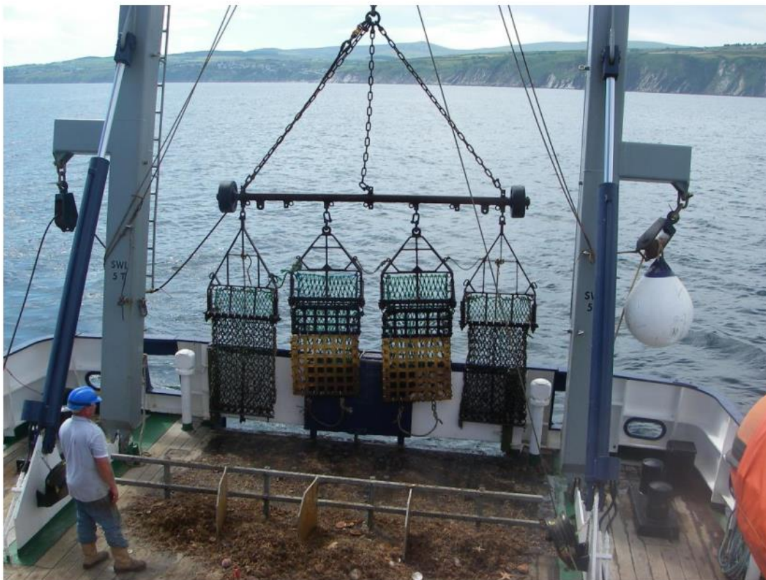
Figure 12 Sea trials of the Oban dredge (centre two dredges) compared with standard spring toothed dredges
