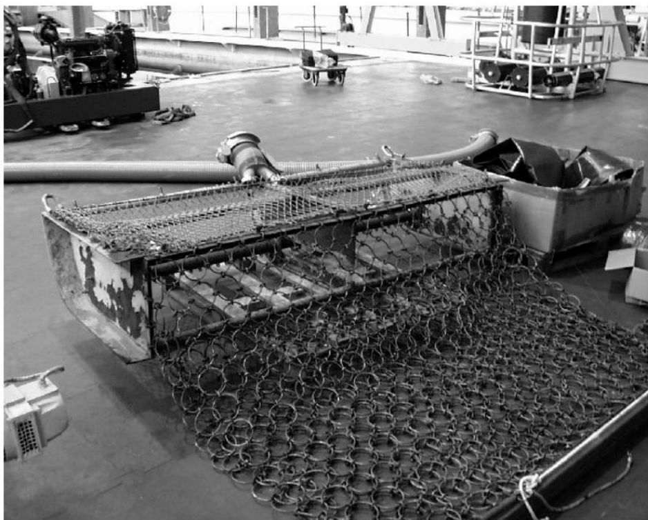
Figure 10 The hydraulic or water jet dredge, designed and built by IFREMER for the Ecodredge project for catching scallops. The angle of the water jets was varied, but mostly set at 45° see Lart ed., (2003)
