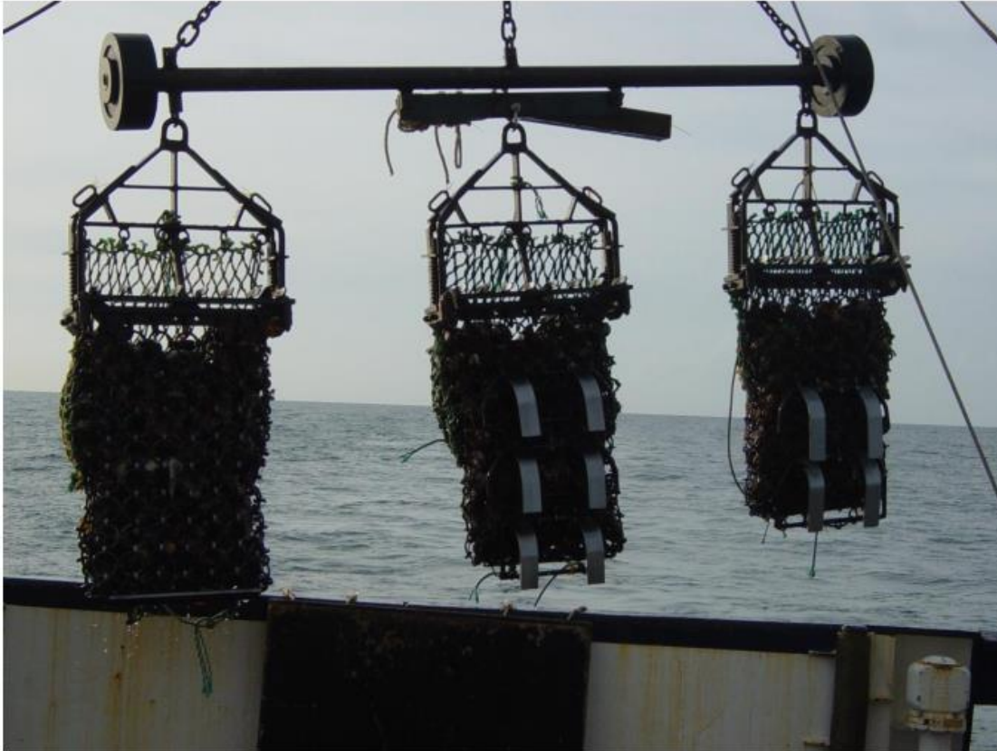
Figure 11 Image of dredges with (from right to left) two and three skids attached, during sea trials. Designed by Ewout Costerus (Cyclone Marine Ltd) and John Coppack (Gannet Marine Ltd). Image: Ewout Costerus.
